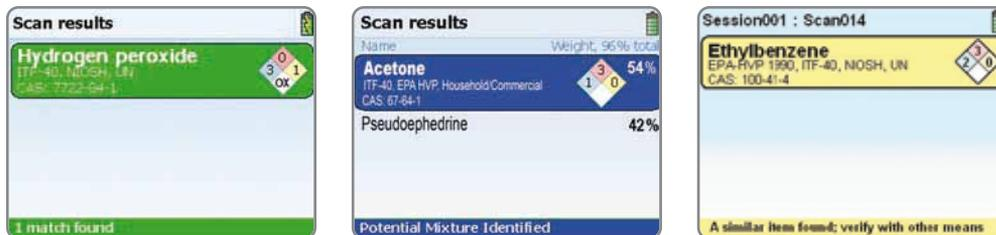
Color-coded result screens require no user interpretation and provide rich content for faster, more informed decision making. Onboard NIOSH and CAMEO guides provide detailed hazard information. Patented chemometric algorithms enable automatic mixture analysis, shown with a blue screen result.
