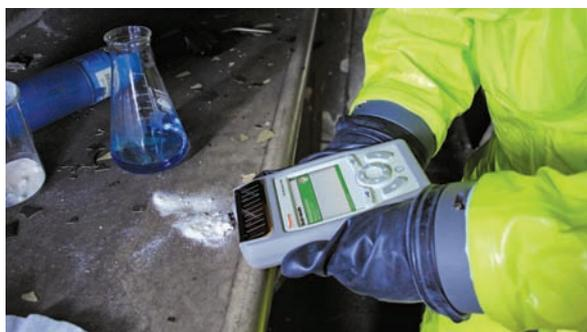
The Thermo Scientific FirstDefender RM instrument is the next generation Raman spectrometer for rapid, accurate identification of unknown chemicals directly in the field. Building on the award-winning, field proven FirstDefender®, significant improvements have been made in speed, performance, mixture analysis and user interface incorporating extensive user feedback and the latest technical advances.
