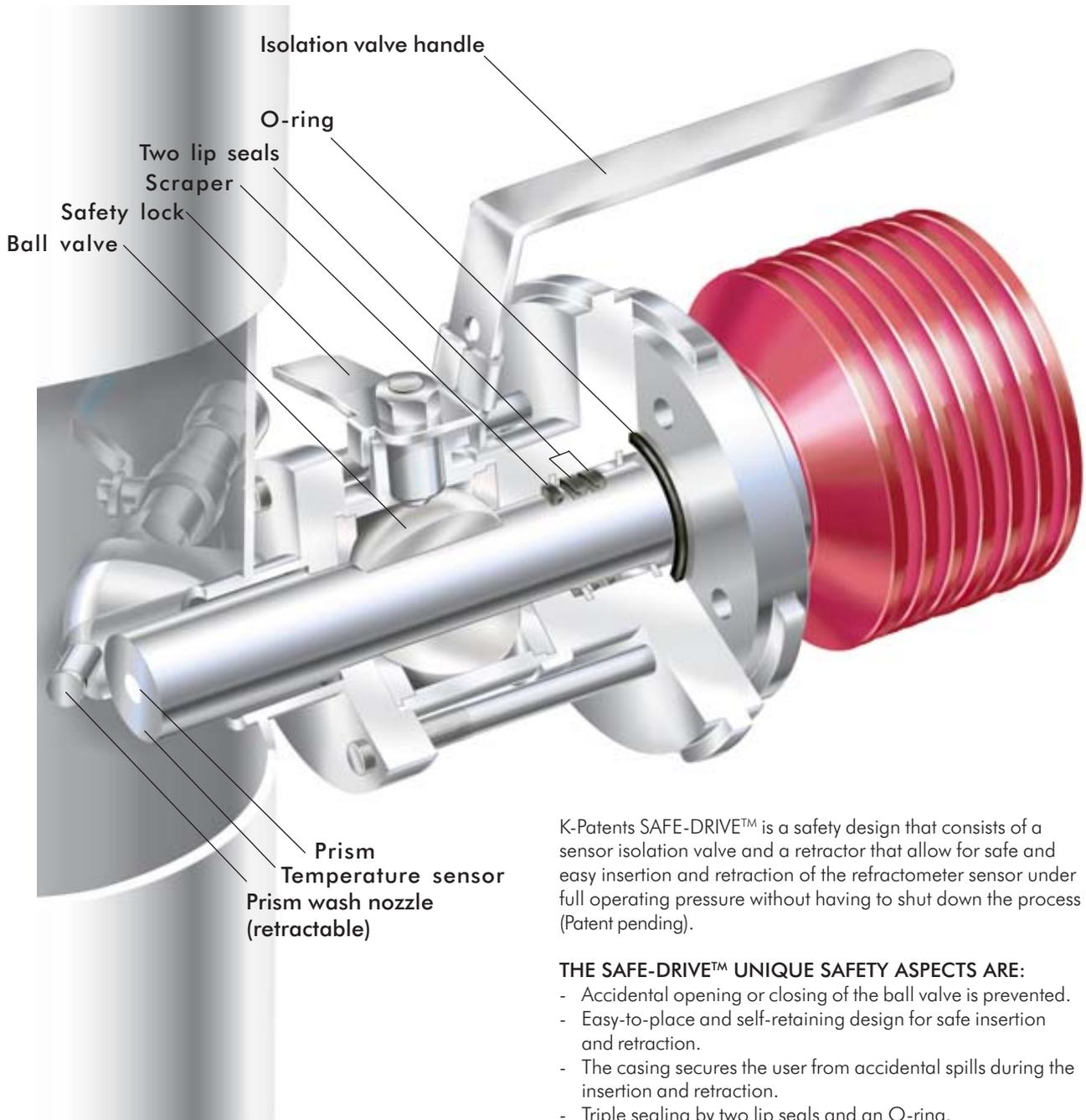
K-Patents SAFE-DRIVE™ is a safety design that consists of a sensor isolation valve and a retractor that allow for safe and easy insertion and retraction of the refractometer sensor under full operating pressure without having to shut down the process (Patent pending).
