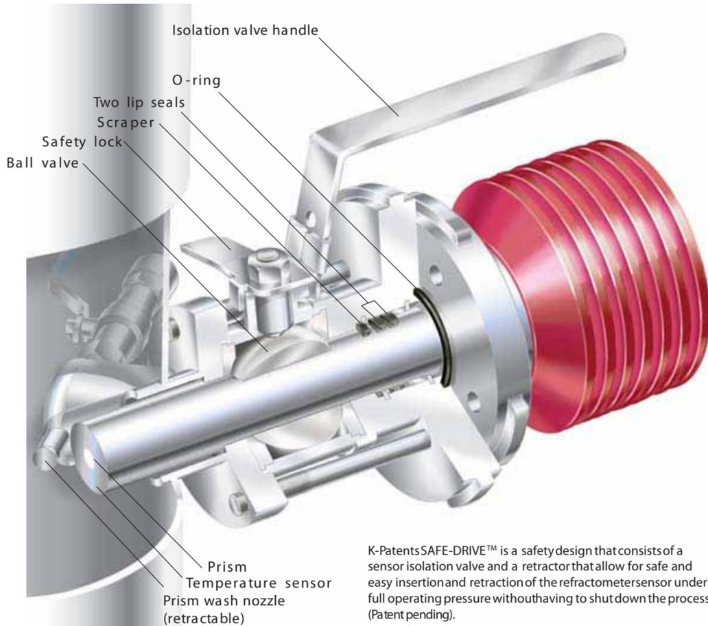
K-Patents SAFE-DRIVE™ is a safety design that consists of a sensor isolation valve and a retractor that allow for safe and easy insertion and retraction of the refractometer sensor under full operating pressure without having to shut down the process (Patent pending).
