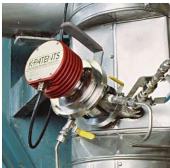
SAFE-DRIVE™ PROCESS REFRACTOMETER PR-23-SD
